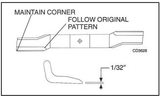
Figure 12. Blade Sharpening
